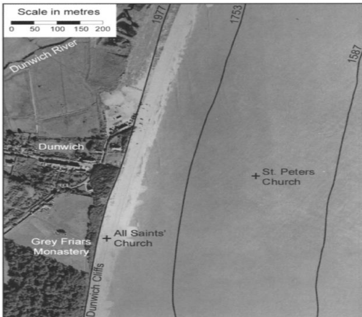
Figure 8. Air photograph of Dunwich taken in 2000, showing positions of the coastline and former churches in 1977, 1753, and 1587. Coastline positions taken from Agas (1587) and Robinson (1980).
